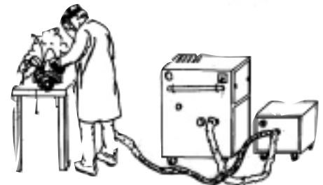
"ON-TOOL CAPTURE" OF GRINDING DUST COMPLETE WITH MOBILE FILTRATION
