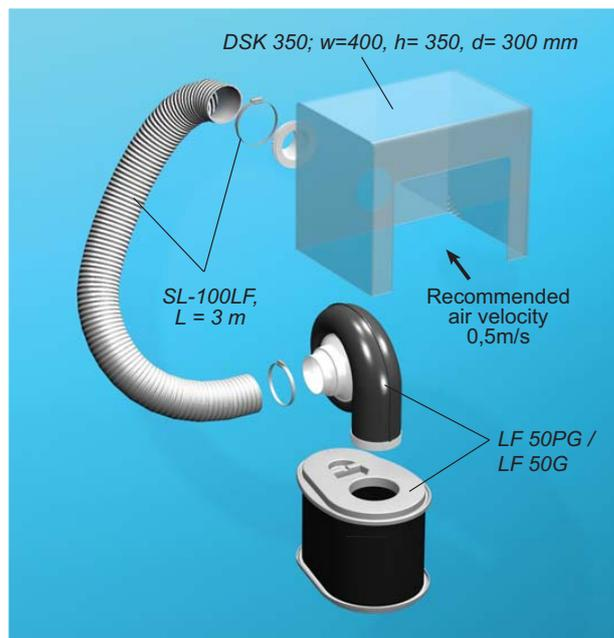
The LFK 350C is a unique system using a polycarbonate cabinet, for maximum peace of mind. When working within the cabinet you are assured that effective capture is always there. Ideal for open glue pots, analytical equipment or test areas.
