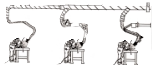
INTERNALLY SUPPORTED EXTRACTION ARM COMPLETE WITH CENTRAL EXHAUST FAN
