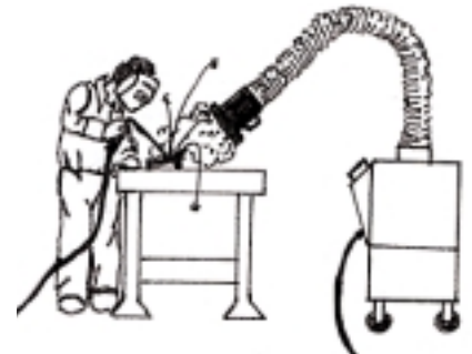
MOBILE FUME EXTRACTION - WELDING
